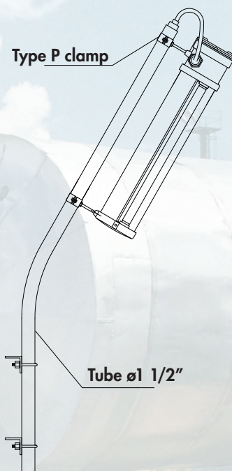
Pole mounting for FLF...L with barrier cable gland
